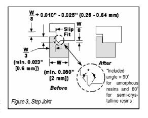
The design of the energy director uses the same basic design thought process used in the butt joint energy director (i.e., material, requirements, part size). Note that a minimum wall thickness of 0.080 inch (2 mm) is recommended for this design.
