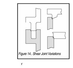
irregular shapes. This is due to difficulty in holding the molding tolerances necessary to obtain consistent results. An energy director type joint would be suggested for parts falling outside of these parameters (i.e., 3.5 inch, sharp corners, irregular shapes).
