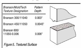
Usually the texture is 0.003 to 0.006 inch deep (0.076 to 0.152 mm), and is varied based on the height of the energy director. In most cases, the advantages include increased weld strength, reduced flash or particulate, reduced weld times, or lower amplitude requirements.
