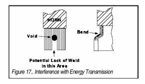
horn contact point to the interface of the parts to be welded, especially in shear.
