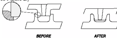
Figure 2.. Stud in Boss or Blind Hole
