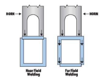
**Near Field Weld (Direct):** Refers to a weld where the contact surface of the horn is 1/4" or less away from the joint surface. It is important that the horn fits exactly the contour of the part to be welded.
