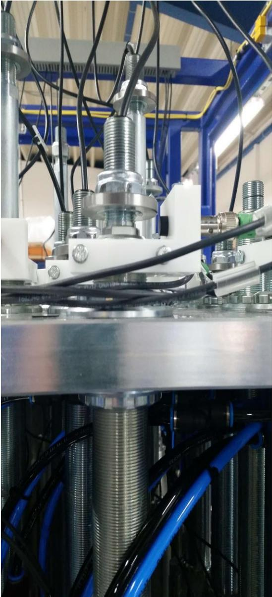
Welding actuators with horns
