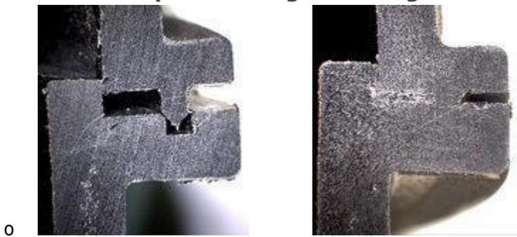
o Unwelded condition      Welded condition
