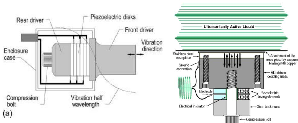
Above ultrasonic welding transducer
