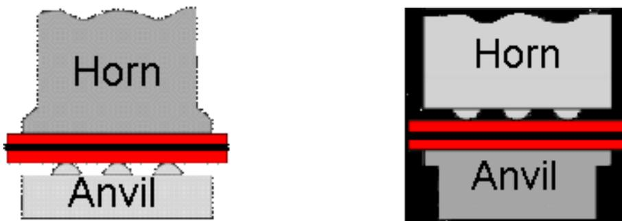
Possibilities of energy focusing due to variations in anvil structures or in the sonotrode / horn
