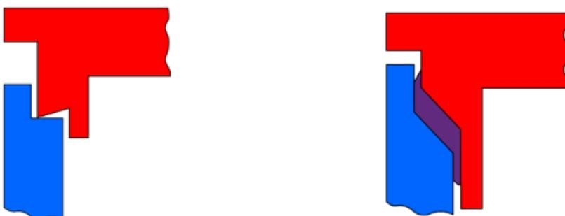
Possibilities of energy focusing due to variations in the joint design / spot welding
