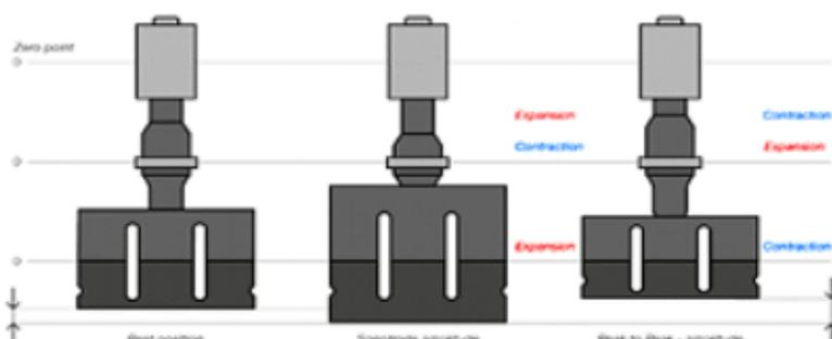
**Schematic diagram of the sonotrode movement**
