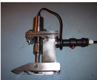
Ultrasonic cutter vibrates its blade 20,000 - 40,000 times per second (20 - 40 kHz). Because of this movement, the ultrasonic cutter can easily cut resin, rubber (tires), nonwoven fabric and composite materials (wind mill wings production).
