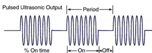
The percentage of time that the ultrasonic energy is on may also be changed to produce varied results. At slower pulse rates, more rapid degassing of liquids occurs as coalescing bubbles of air are given an opportunity to rise to the surface of the liquid during the time the ultrasonic energy is off. At more rapid pulse rates, the cleaning process may be enhanced as repeated high energy "bursts" of ultrasonic energy occur each time the energy source is turned on.
