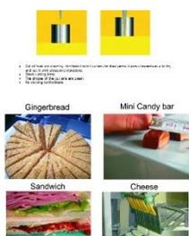
Ultrasonic food cutting is a process utilizing ultrasonic titanium knives that vibrate at frequencies from 20 to 40 kHz. Applying ultrasonic vibration to a cutting tool creates a nearly frictionless cutting surface which provides many benefits.
