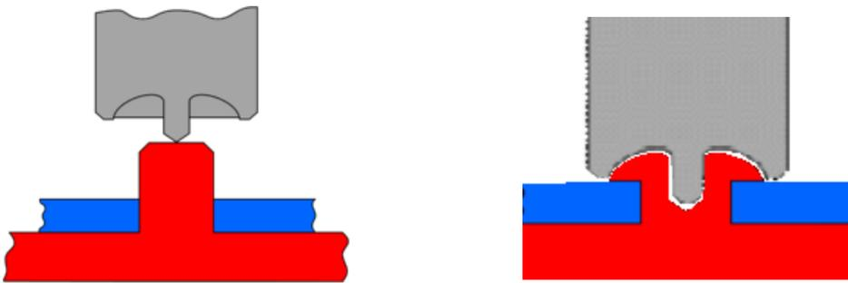
Focusing by the **sonotrode / horn shape** (weld tool); e.g. during the ultrasonic staking process, the sonotrode assumes the task of energy concentration. The centering tip serves as melting initiation aid.
