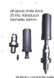
Each object has its special frequency, by which the object is stable and easy to oscillate. By adding an external force that corresponds to that special frequency, a small force can obtain a large oscillation. This phenomenon is called resonance. The cutting edge is oscillated greatly with the use of resonance.
